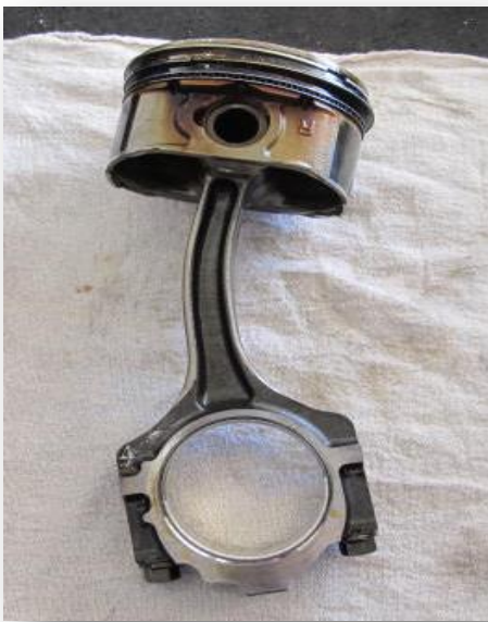
Figure 8: Bent Connecting Rod from Hydro lock
