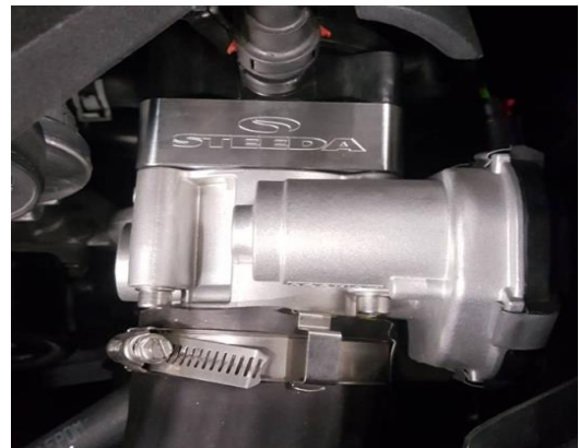
Figure 16D: Aftermarket Air Induction setup
