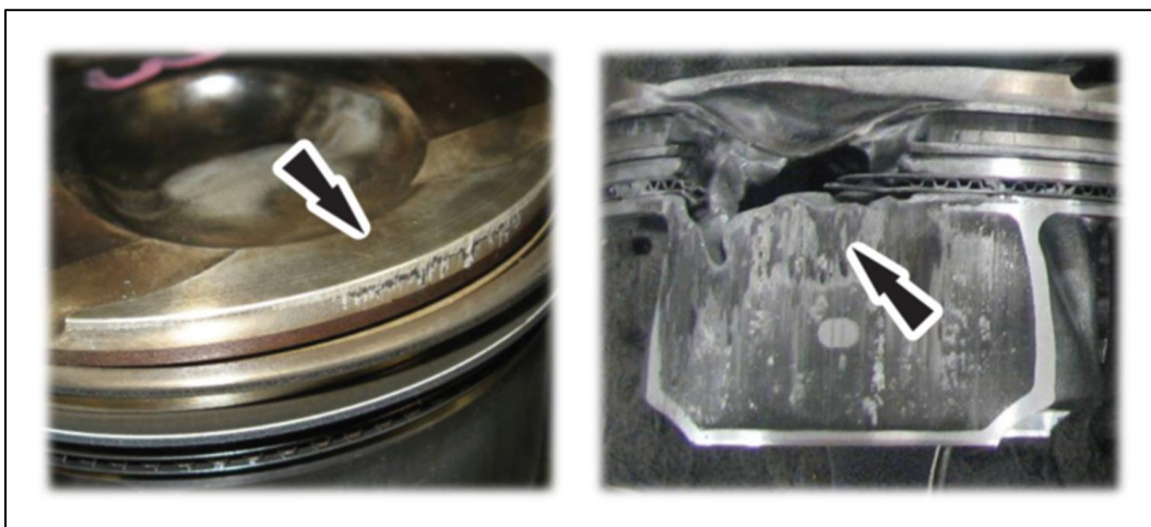
Figure 4: Light/Heavy Knock Damage
