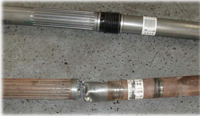
Figure 11A: Twisted Driveshaft
