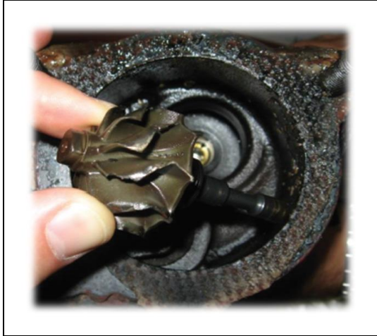
Figure 12: Compressor Blade Damage from Overspeed Event
