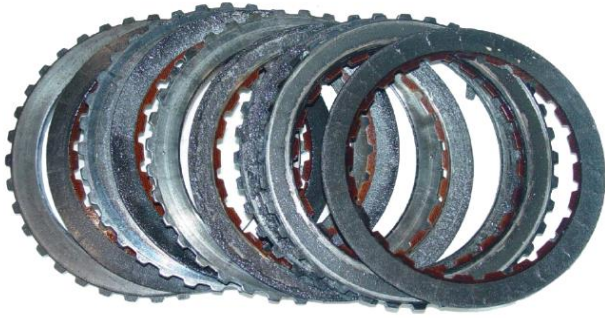
Figure 10A: Damaged Clutch Discs
