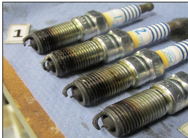
Figure 7B: Spark Plug Damage and Abnormal Color
