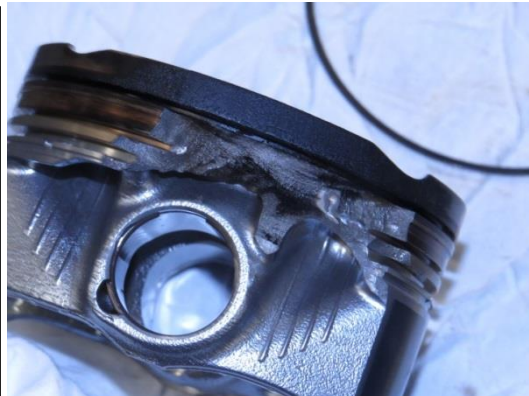
Figure 3: Piston Ring Land Damage
