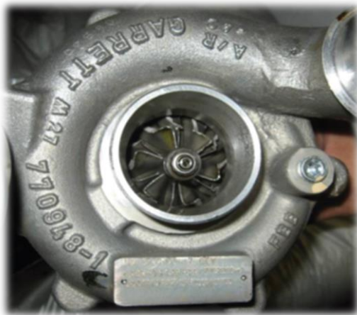
Figure 13: Compressor Blade Damage from Overspeed Event
