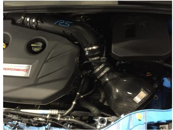
Figure 16B: Aftermarket Air Filter Setup
