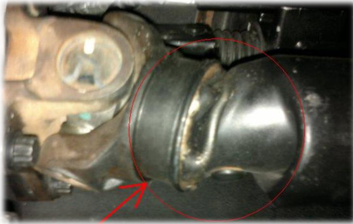
Figure 11B: Twisted Driveshaft
