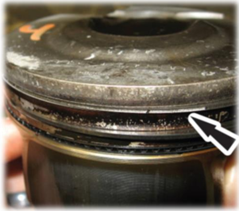
Figure 6A: Piston Ring Damage
