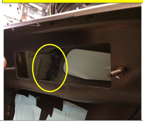
The Passenger side Exterior Cowl Top Baffle area can be accessed by removing the PCM. Make sure the Baffle is properly sealed.
