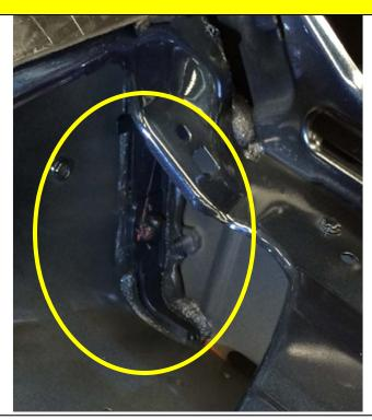
The Driver side Exterior Cowl Top Baffle area can be accessed by removing the cowl top leaf screen and wiper arms. Make sure the Baffle is properly sealed.
