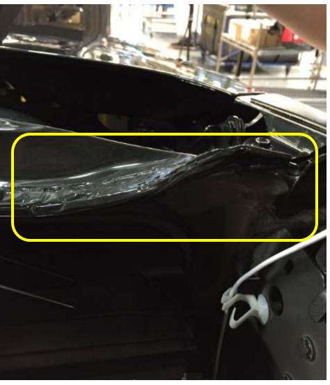
The Cowl Top Tape can be accessed by removing the interior A-pillar trim panel. Make sure the tape is not damaged and is properly sealing.
