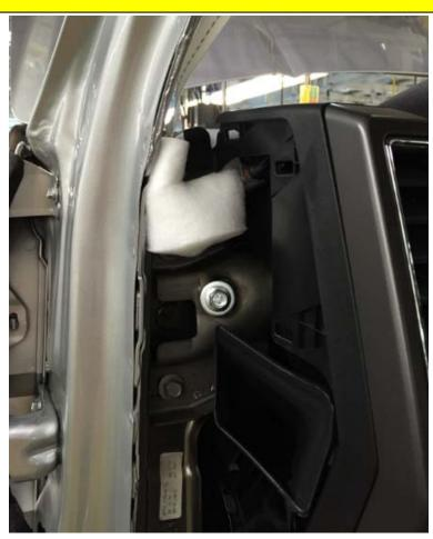
Foam stuffer blocks should be located between the IP and A-pillar.
